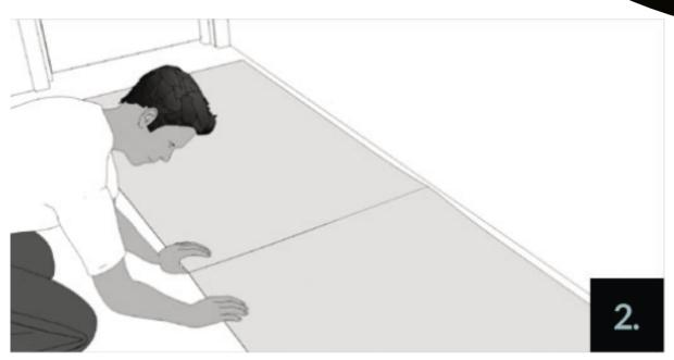
2.1 Next, knowing the sheet format, we shall mark the width and height measurements on the wall, to assist with its installation later. Cam/ out the construction layout, depending both on the wall the design and the use demands. Determine type and color of placement joints, cuts, and perimeter joints
